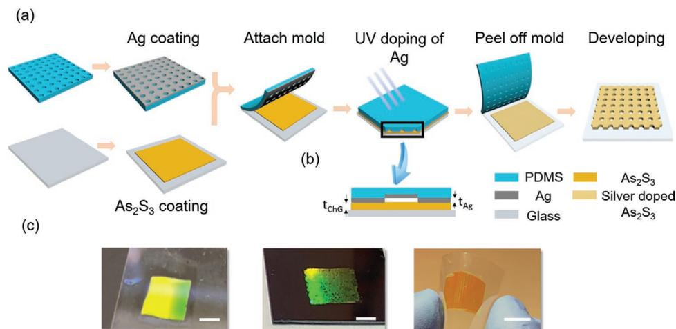
**Figure 1.** IL-SD fabrication process. a) Schematic process flow of using an Ag-coated PDMS stamp to generate patterns in an  $\text{As}_2\text{S}_3$  film. b) Illustration showing the photodoping of Ag through the interface between the  $\text{As}_2\text{S}_3$  film and the Ag-coated PDMS stamp into the  $\text{As}_2\text{S}_3$  film. c) Photograph of the fabricated ChG nanostructures on glass (left), silicon (center), and plastic (right) substrates, respectively. Scale bars represent 1 cm.
