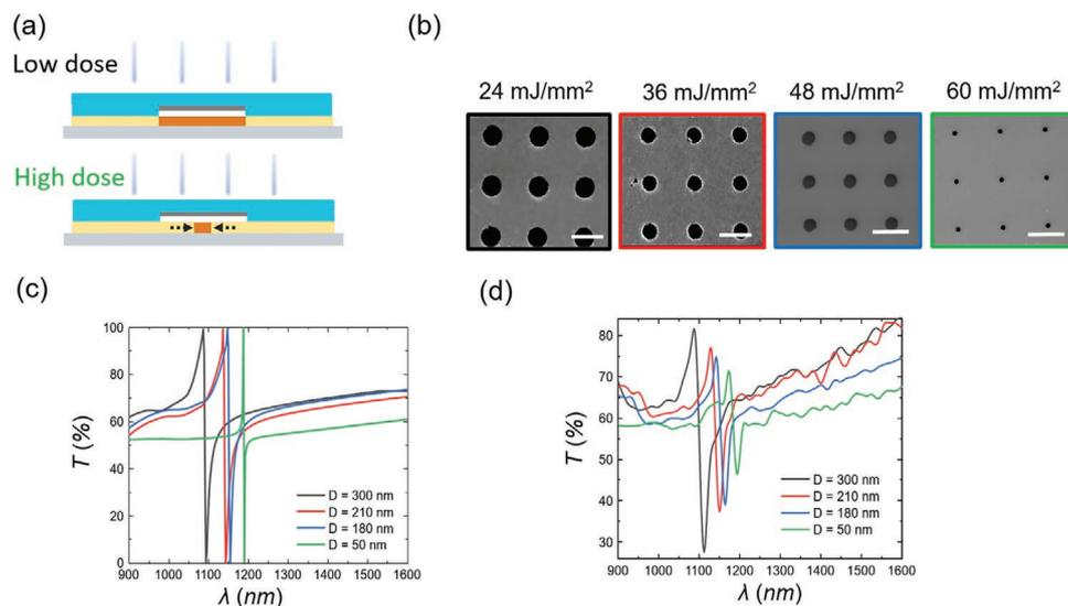
**Figure 6.** Tuning the pattern size and the optical resonance of the  $\text{As}_2\text{S}_3$  PhC via controlled lateral diffusion of Ag. a) Schematic of the lateral diffusion during the photodoping of Ag. b) SEM images of 2D nanohole arrays with the hole diameter ranging from 300 to 50 nm. These patterns are formed based on a single PDMS stamp. Scale bars represent 500 nm. c) Simulated and d) measured transmission spectra of the obtained 2D nanohole arrays shown in (b).
