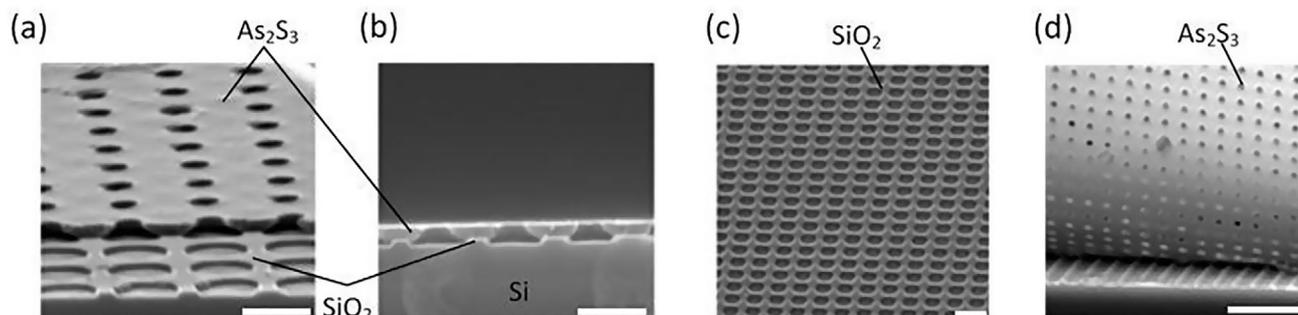
**Figure 3.** SEM images of using a ChG-based mask to transfer patterns from the ChG film to the substrate beneath it. a) Prospective and b) cross-sectional view of the ChG-SiO<sub>2</sub>-Si structure after a 10 s over-etching. c) Top view of the SiO<sub>2</sub> pattern after removal of ChG. Scale bars represent 500 nm in (a–c) and 3  $\mu$ m in (d).
