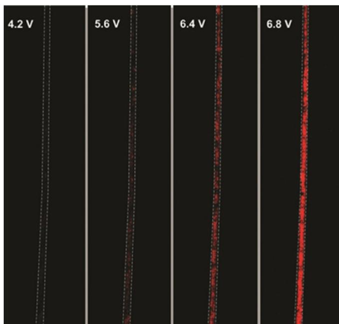
**Figure 2.** Luminescence responses of the fabricated nanofiber to different voltages applied.
