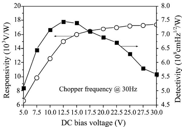
Fig. 11. Dependence of the responsivity and detectivity on the dc bias voltage.
