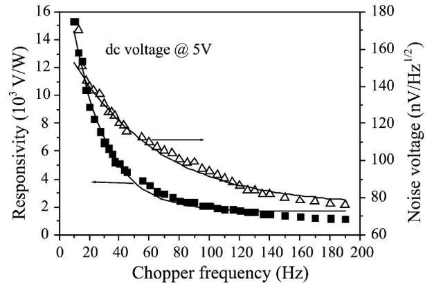
Fig. 9. Dependence of the responsivity and noise voltage on the chopper frequency.
