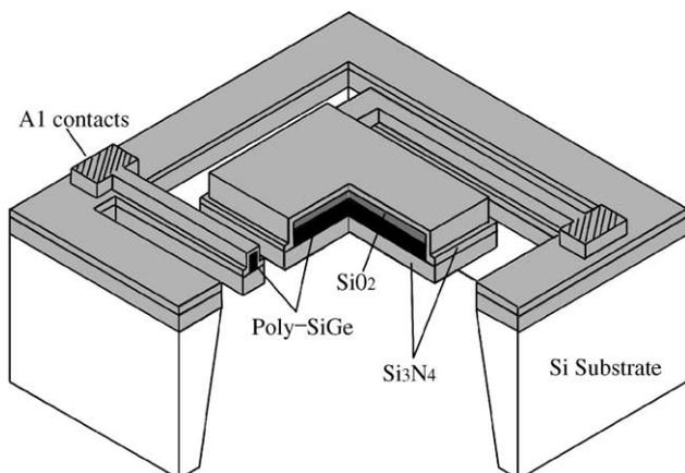
Fig. 6. Schematic diagram of the poly-SiGe microbolometer.
