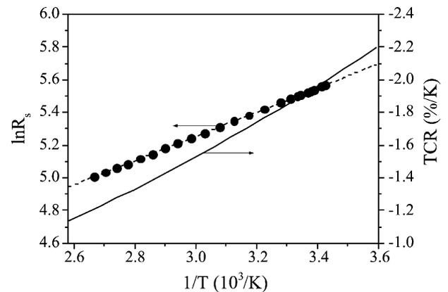
Fig. 4. Dependence of the resistance and TCR on the operating temperature.
