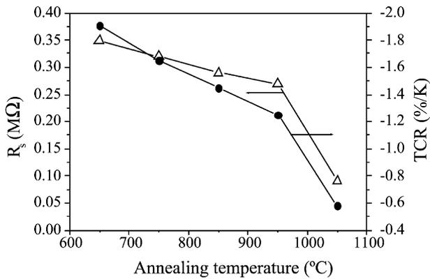
Fig. 5. Dependence of the resistance and TCR on the annealing temperature.
