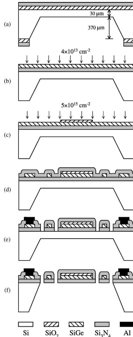
Fig. 7. Main fabrication process of the poly-SiGe microbolometer.
