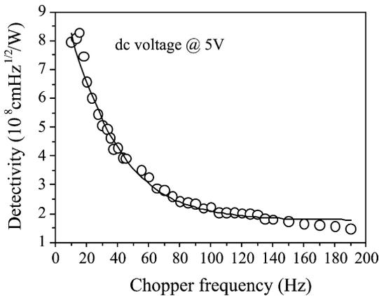
Fig. 10. Dependence of the detectivity on the chopper frequency.
