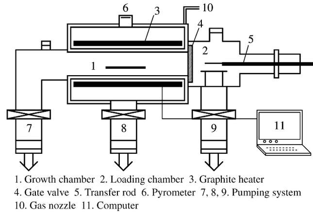
Fig. 1. Schematic diagram of the UHV/CVD system.
