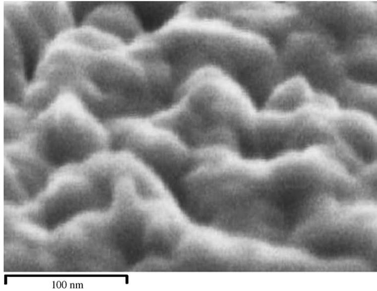
Fig. 2. SEM surface morphology of the poly-SiGe film.
